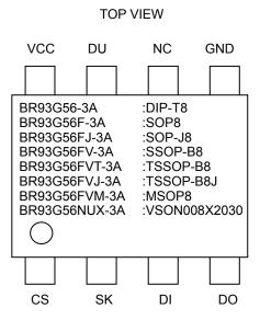
Figure 3. Pin Configuration
