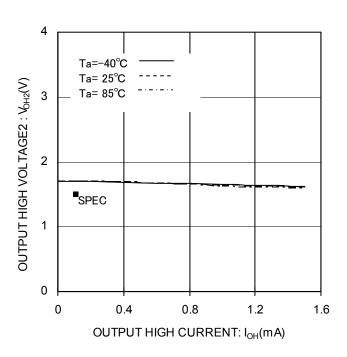
Figure 9. Output High Voltage2 vs Output High Current (Vcc=1.7V)
