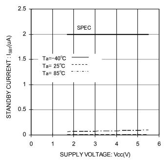
Figure 20. Standby Current vs Supply Voltage (CS=0V)
