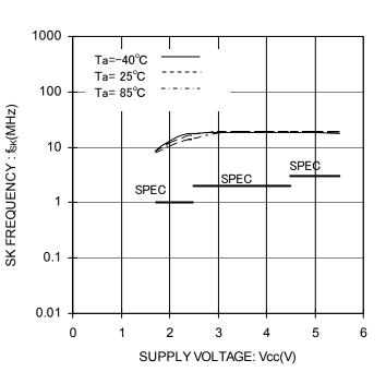
Figure 21. SK Frequency vs Supply Voltage
