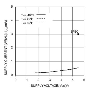
Figure 19. Supply Current (WRAL) vs Supply Voltage (f<sub>SK</sub>=3MHz)
