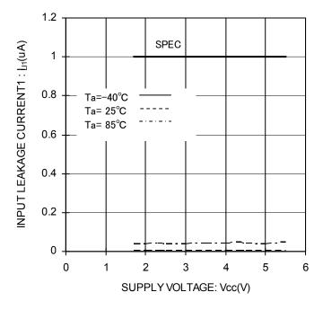
Figure 10. Input Leakage Current1 (CS) vs Supply Voltage
