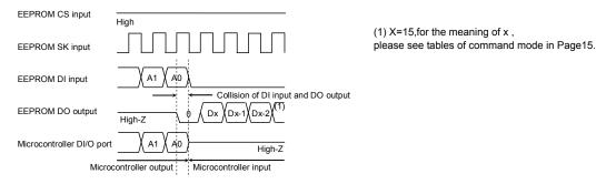
Figure 50. Collision Timing at Read Data Output at DI, DO Direct Connection
