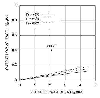
Figure 6. Output Low Voltage1 vs Output Low Current (Vcc=2.7V)
