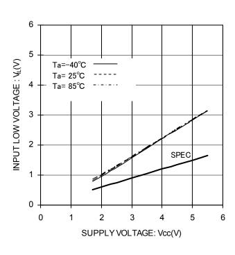
Figure 5. Input Low Voltage vs Supply Voltage (CS,SK,DI)
