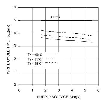
Figure 33. Write Cycle Time vs Supply Voltage
