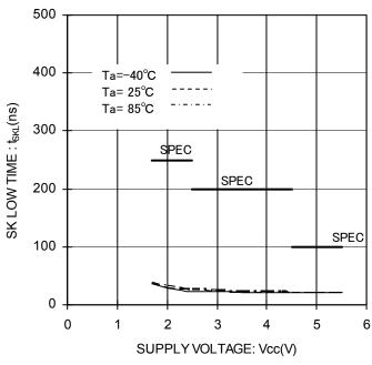
Figure 23. SK Low Time vs Supply Voltage
