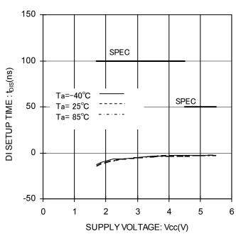
Figure 27. DI Setup Time vs Supply Voltage
