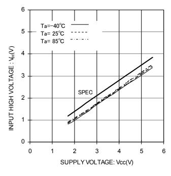
Figure 4. Input High Voltage vs Supply Voltage (CS,SK,DI)
