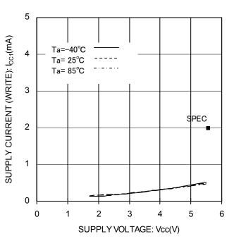
Figure 14. Supply Current (WRITE) vs Supply Voltage  $(f_{SK}=1MHz)$
