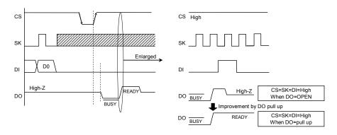
Figure 45. READY Output Timing at DO=OPEN
