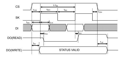
Figure 1. Serial Input / Output Timing
