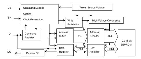
Figure 2. Block Diagram
