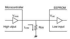
Figure 44. CS Pull Down Resistance
