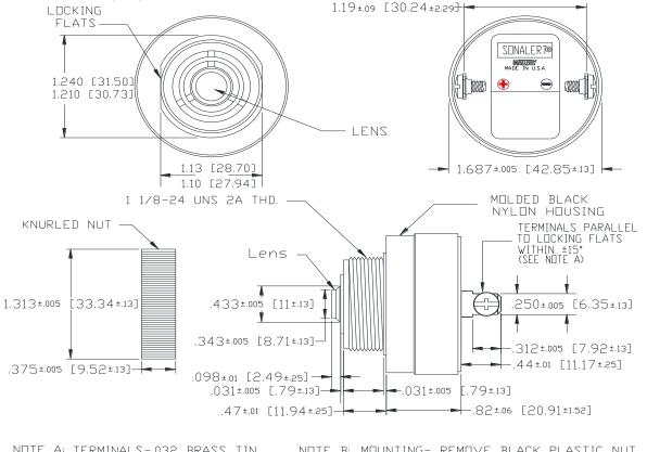
NOTE A: TERMINALS-.032 BRASS TIN PLATED, TAPPED FOR #6-32 SCREW. TWO #6-32 NI PLATED BRASS SCREWS TWO #6-32 NICKEL INCLUDED. WILL ACCEPT 1/4" QUICK CONNECT.
