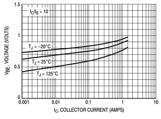
Figure 7. Base-Emitter Saturation Region
