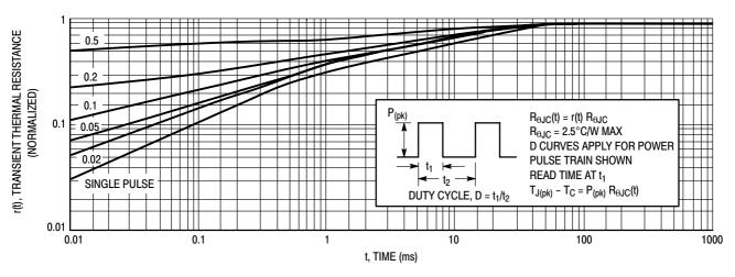
Figure 24. Typical Thermal Response ( $Z_{\theta JC}(t)$ ) for BUH51
