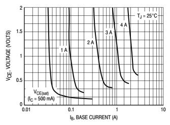
Figure 8. Collector Saturation Region
