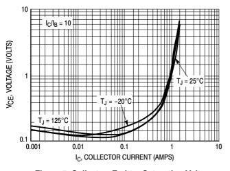
Figure 5. Collector-Emitter Saturation Voltage
