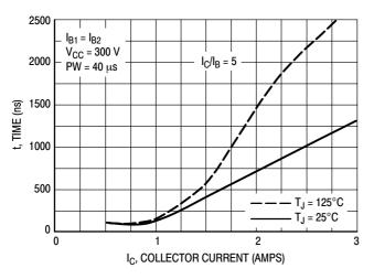
Figure 11. Resistive Switching, ton
