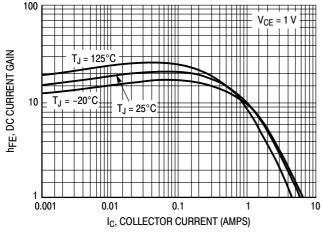
Figure 1. DC Current Gain @ 1.0 V
