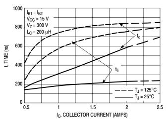
Figure 15. Inductive Storage Time,  $t_c \& t_{fi} @ I_C/I_B = 10$
