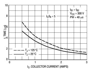
Figure 12. Resistive Switch Time, toff
