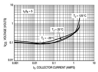
Figure 4. Collector-Emitter Saturation Voltage
