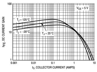
Figure 3. DC Current Gain @ 5.0 V
