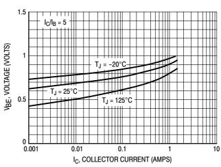
Figure 6. Base-Emitter Saturation Region
