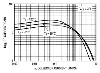
Figure 2. DC Current Gain @ 3.0 V
