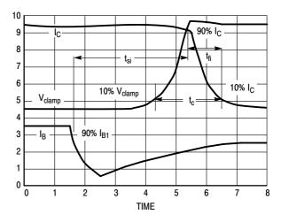
Figure 19. Dynamic Saturation Voltage Measurements
