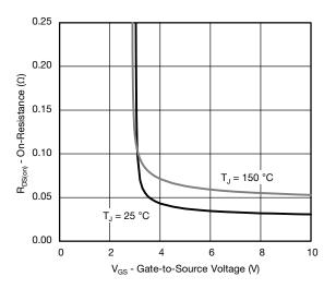
On-Resistance vs. Gate-to-Source Voltage
