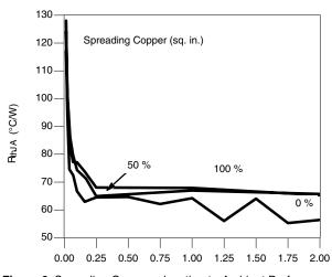
Figure 6. Spreading Copper - Junction-to-Ambient Performance
