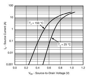
Source Drain Diode Forward Voltage
