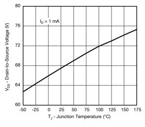
Drain Source Breakdown vs. Junction Temperature
