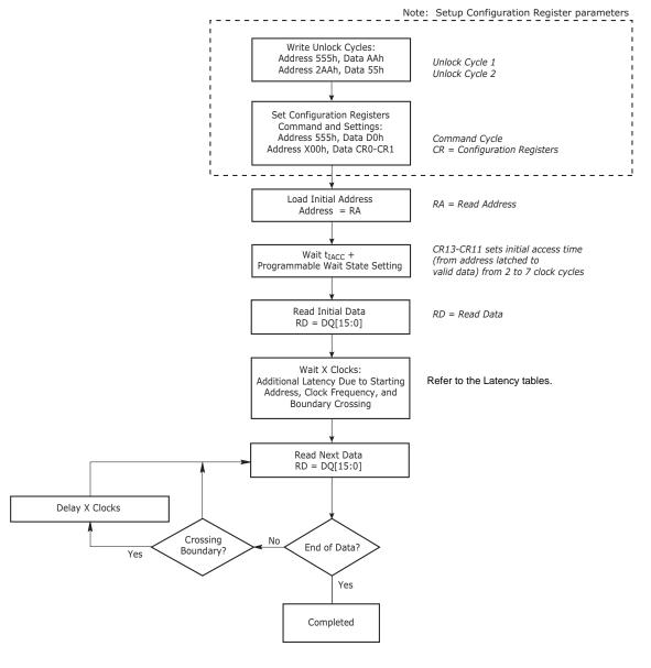
Figure 7.1 Synchronous Read Flow Chart
