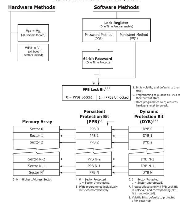
Figure 8.1 Advanced Sector Protection/Unprotection
