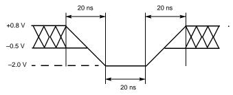
Figure 11.2 Maximum Positive Overshoot Waveform
