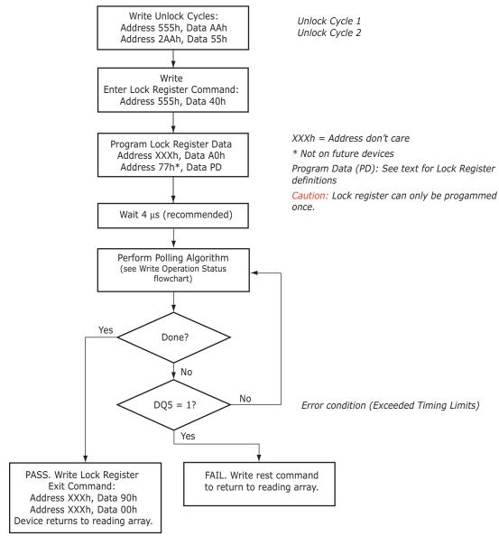
Figure 8.3 Lock Register Program Algorithm
