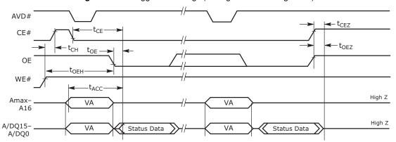
Figure 11.16 Toggle Bit Timings (During Embedded Algorithm)
