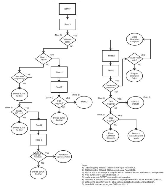
Figure 7.5 Write Operation Status Flowchart
