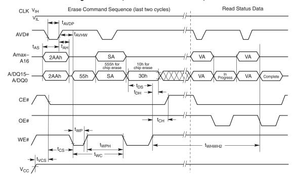
Figure 11.13 Chip/Sector Erase Command Sequence
