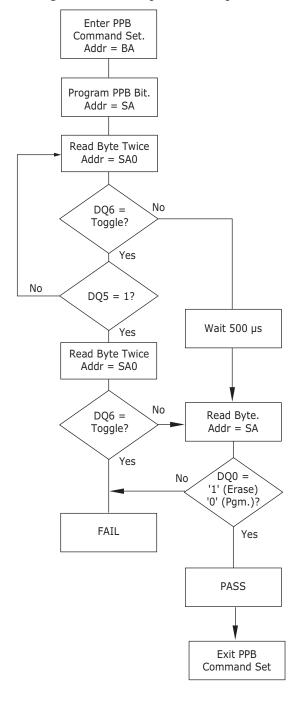
Figure 8.2 PPB Program/Erase Algorithm
