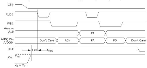
Figure 11.14 Accelerated Unlock Bypass Programming Timing
