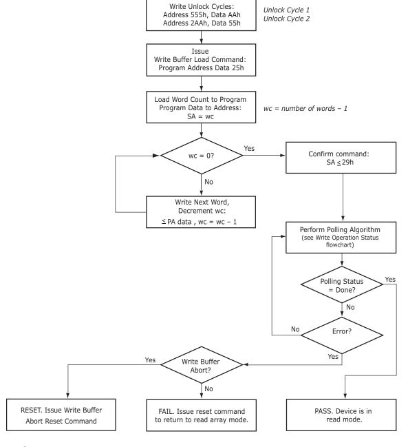
Figure 7.3 Write Buffer Programming Operation
