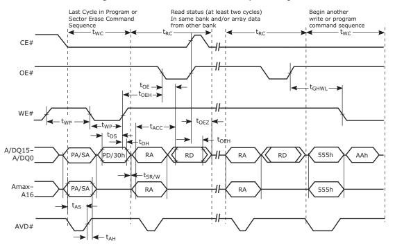
Figure 11.21 Back-to-Back Read/Write Cycle Timings
