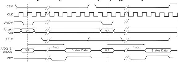
Figure 11.17 Synchronous Data Polling Timings/Toggle Bit Timings
