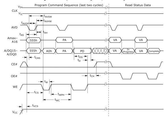
Figure 11.12 Asynchronous Program Operation Timings
