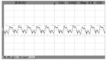
Step Load Transient Response (Vin=12V, Vout=2.5V, Cload=0, lout=1.5A to 3A)
