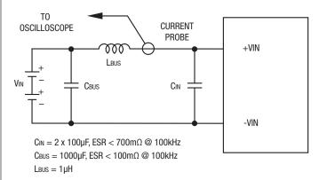
Figure 4. Measuring Input Ripple Current
