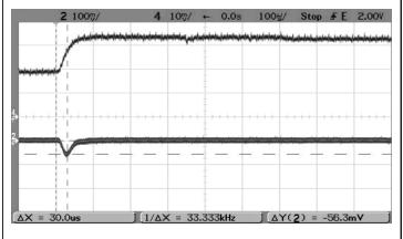
Step Load Transient Response (Vin=12V, Vout=2.5V, Cload=0, lout=3A to 1.5A)
