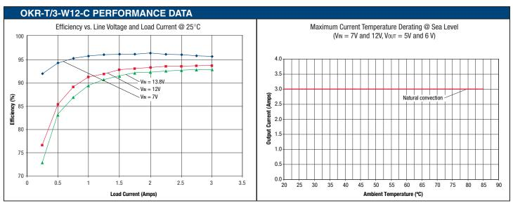
There is no derating for Vout = 0.591V. to 5.5V. at full load.
