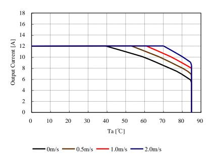
The above derating limits apply to this product soldered directly to 101.6\*180mm\*1.6mm PCB (double-sided, with 70um copper). Any adjacent parts of high temperature may cause overheating. For reliable operation, please ensure that the FET temperature of this product is maintained below 120°C and the inductor t emperature is below 106°C.
