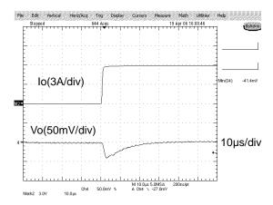
Fig. 12-1. Load Transient Response
