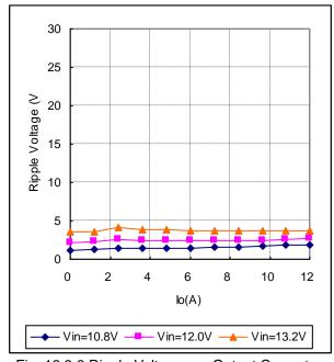
Fig. 12.3.6 Ripple Voltage v.s. Output Current
