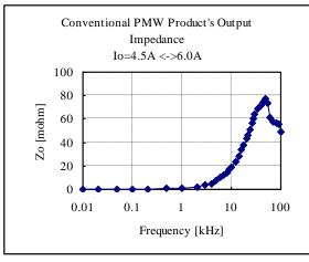
Fig. 12.2.1 Output Impedance of MPDRX003S
