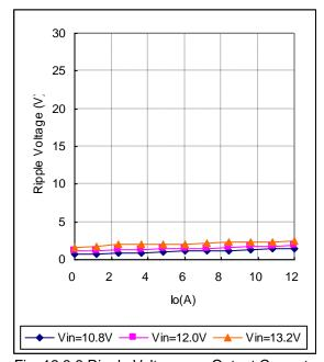
Fig. 12.3.3 Ripple Voltage v.s. Output Current
