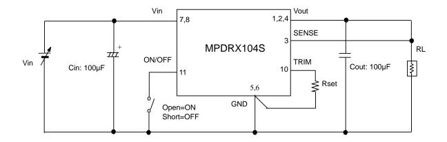
Cin : 100uF / 16V (16ZL120MMRKTA6.3X11,Rubycon) (Low-impedance Electrolytic Capacitor) Cout : 100uF / 6.3V (GRM32EB30J107ME16L, Murata)
