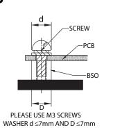
THE DISTANCE BETWEEN CUSTOMER PLATE AND TOP OF THE POWER SUPPLY L  $\geq$ 4mm; IF L  $\leq$ 4mm, ISOLATION FILM OR MYLAR WILL BE NEEDED
